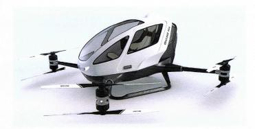
Chinese manufacturer Ehang has unveiled the world's first passenger-carrying drone, which will transport individuals through the air without a pilot (+ movie). The Ehang 184 drone measures around 1.4 metres high, and features eight propellers held on four arms that can be folded into the vehicle's body for storage. Ehang has called the vehicle the "safest, smartest and eco-friendly low-altitude autonomous aerial vehicle aiming on providing medium-short distance transportation solutions".
